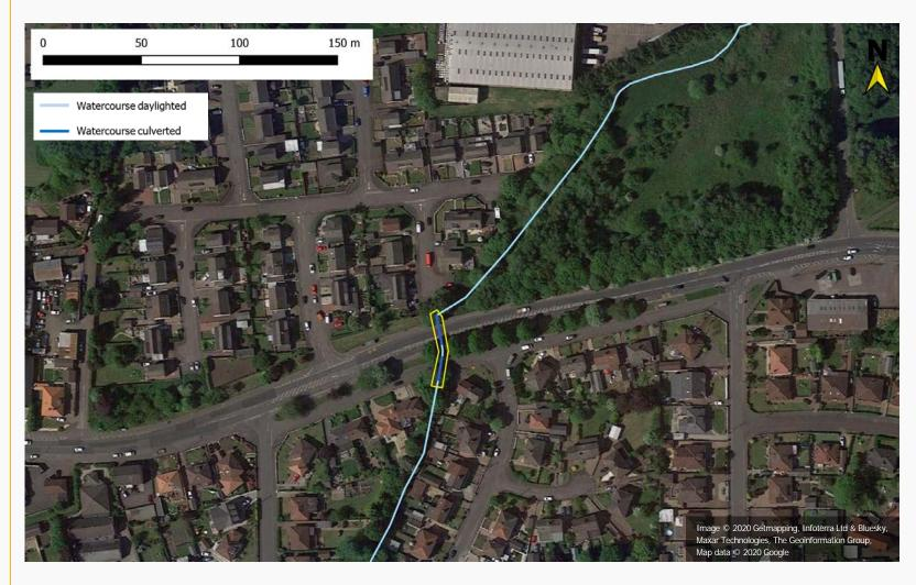
Sediment removal from the road culvert with renovation beneath Baillieston Road will improve the watercourse capacity.
