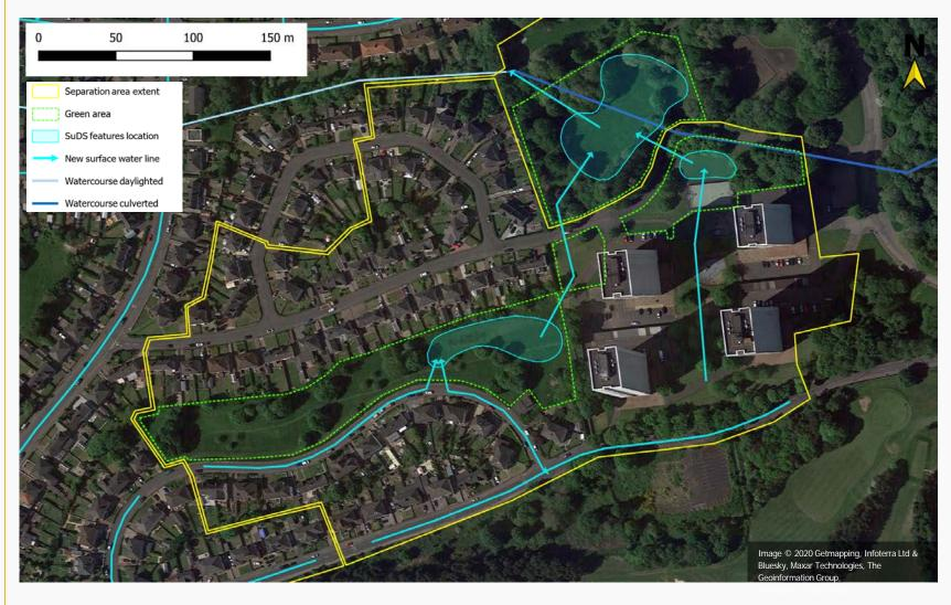
Proposal is a new surface water drainage system to collect runoff from roofs and roads around Comrie Street/Sandyhills Road, Strowan Street and Sandyhill Housing association flats.
