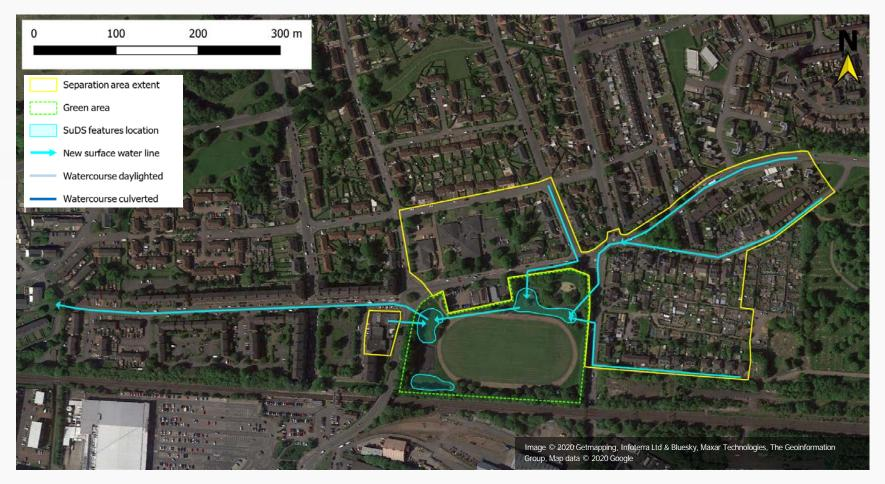
Proposal is a new surface water drainage system to collect runoff from roofs and roads to the north, Day centre buildings, and east around Gartocher Terrace, Hallhill Road and Mansionhouse Drive.
